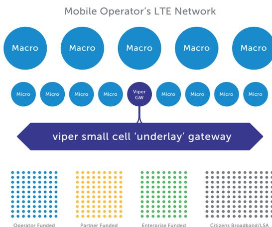
The Viper platform features fully virtualised gateways handling AP security, access control, core network interfacing and network operation. The Viper gateways can be hosted in the Mobile Operator's premises, in an offsite data centre, or cloud hosted.
