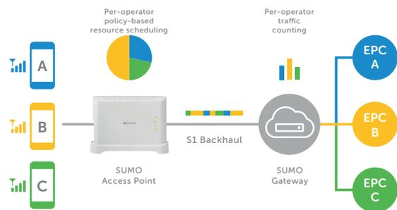
With SUMO, the AP broadcasts multiple PLMN codes on the same spectrum, and all users see the AP as a cell within their home network. A policy based resource scheduler in the AP allocates capacity and bandwidth according to predefined rules. The Viper gateway securely routes all traffic to the appropriate core network for each operator, and traffic counters allow the traffic to be monetised.
